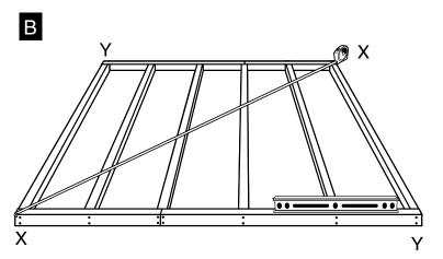
B: Completed Floor Frame should be positioned at building site, leveled, using shims between floor frame and ground before proceeding to Floor Panel Attachment.
